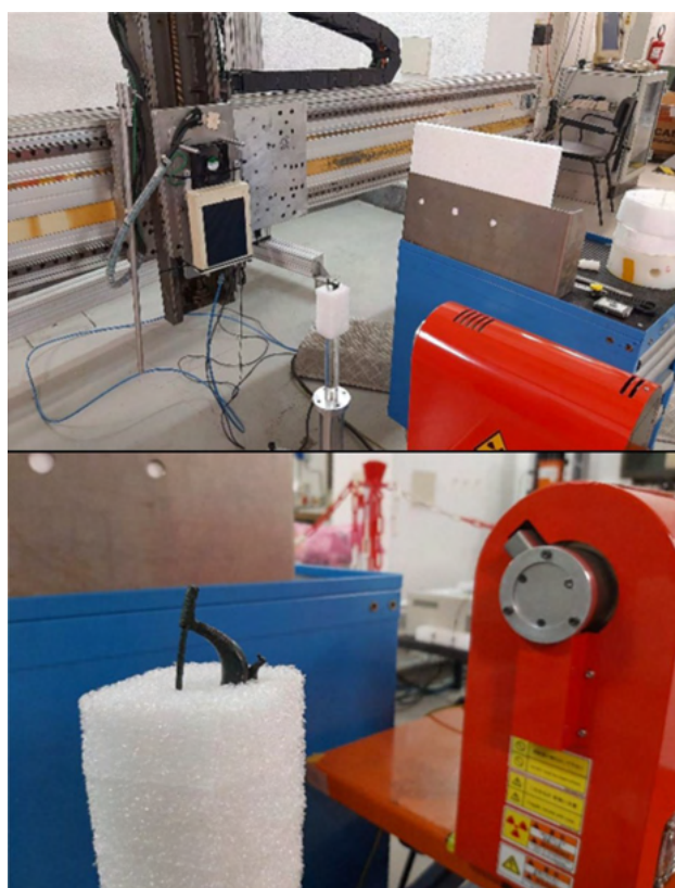
Figure 97. Setup of radiographic analysis and detail of the artefact under investigation.
