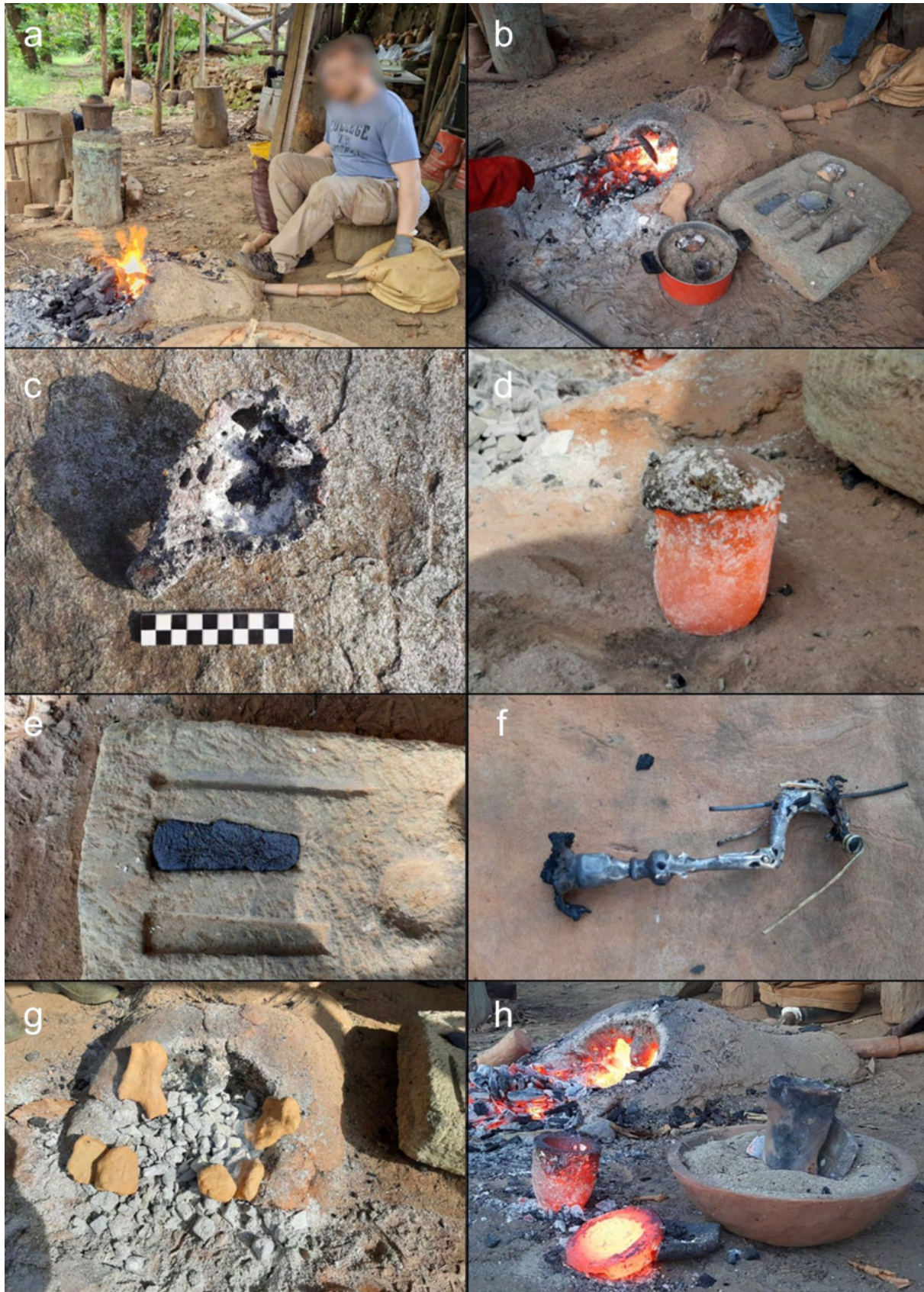
Figure 209. a) Two bellows melting furnace; b) Two bellows melting furnace; c) Ceramic crucible after a bronze casting; d) Graphite crucible with ceramic cap, after casting; e) Bronze ingot; f) Fibula with non-uniform colouring for direct realisation, without preliminary ingot: test specimen 19; g) Heating the moulds on the furnace during casting; h) Vertical positioning of the mould after casting (right); furnace (background); graphite crucible and metal cup (left).
