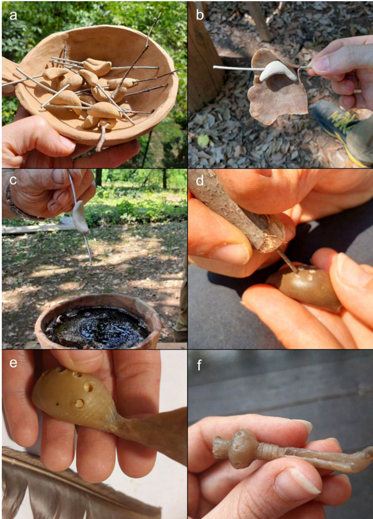
Figure 207. a) Clay cores; b) Coating a clay core with a wax sheet; c) Immersion of a clay core in a liquid wax bath; d) Making the circular decoration with a metal punch; e) Making the circular decoration with a feather; f) Foot modelling.
