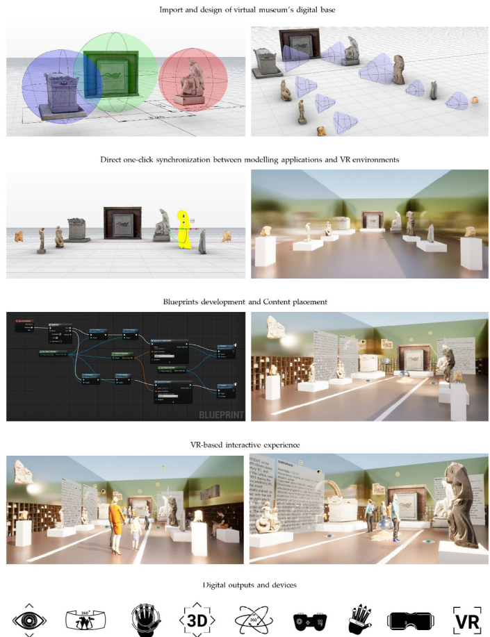
Figure 4. The development process applied to the digital interactive representation of the virtual museum: from textured models to the VR headset in Banfi, et al, 2023.
