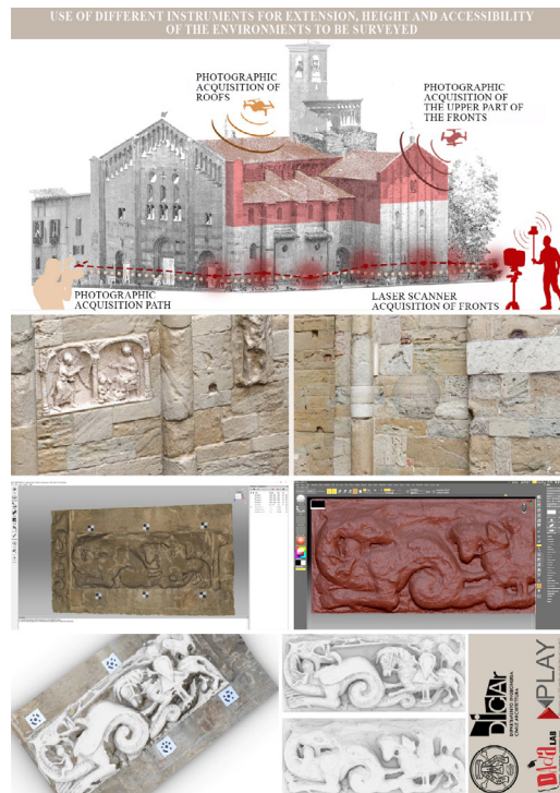
Figure 1. Digitization process of the tile of Saint Giorgio and the Dragon of San Michele Church, Pavia, 2022, DAdA-LAB, DICAr, University of Pavia. Above: integrated survey methodology of St. Michael's Church; middle: detail of photogrammetric models of the facade; bottom: digital and 3D-printed reconstruction of the tile of St. George and the Dragon. Project managers: Prof. Sandro Parrinello, Prof. Marco Morandotti. Research team: Prof. Francesca Picchio, PhD. Silvia La Placa, PhD Student Elisabetta Doria, Research Fellow Hangjun Fu, Research Fellow Alessia Miceli, Intern Alberto Pettineo. Image processing: Silvia La Placa.
