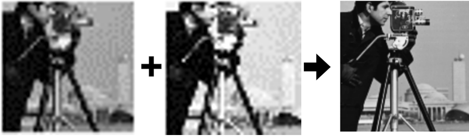
Figure 5.2 Super-resolution is referred to the process to combine multiple low quality images to reconstruct an image of the underlying high-resolution scene.
